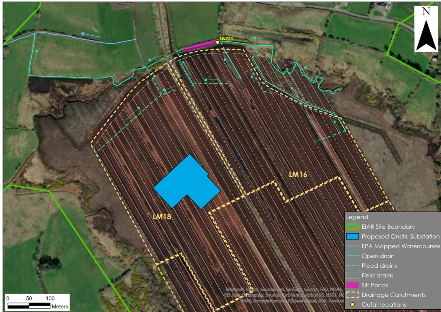
Figure 9-7: EPA Drainage Mapping at Proposed Grid Connection infrastructure under the existing OHL
