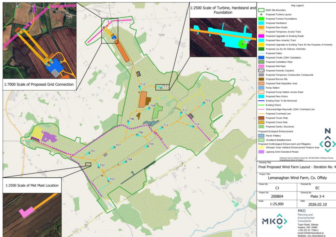
Plate 3-4 Proposed Wind Farm Layout Iteration No. 4 – Final Proposed Wind Farm Layout
