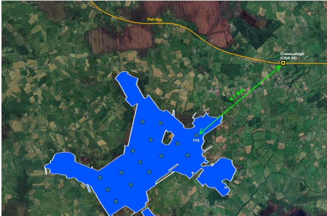
Figure 10. Nearest turbine to Irish Rail GSM-R Basestaion
