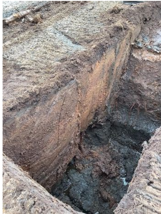
Plate 2: TP 1 after peat excavation
