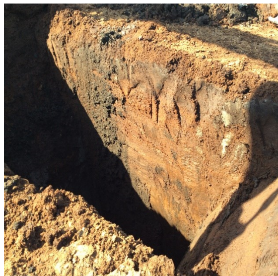
Plate 2: TP 1 after excavation
