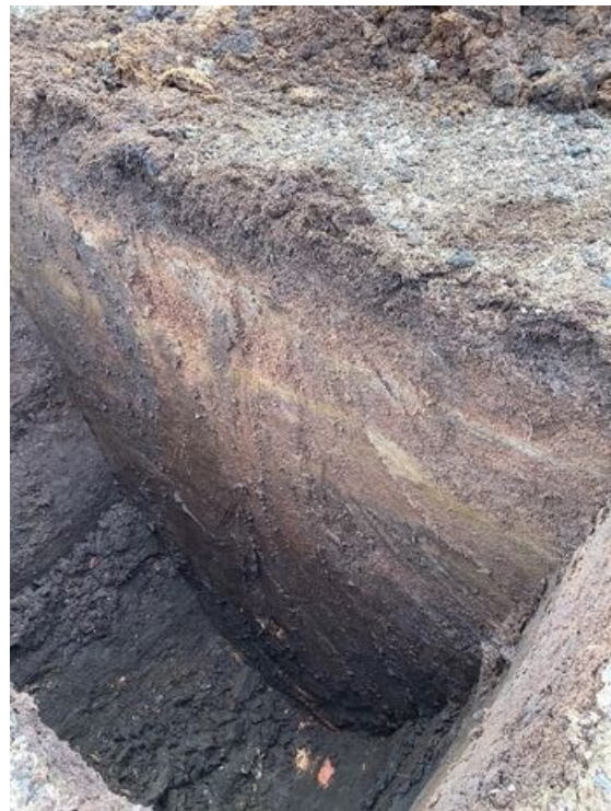
Plate 14: TP7 after peat excavation
