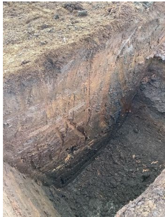
Plate 46: TP23 after peat excavation
