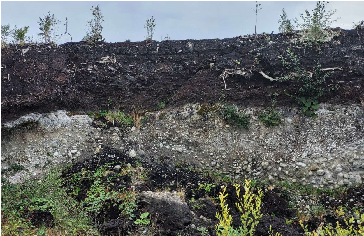
Figure A-4 Soil Profile of Peat overlying Glacial Till.
